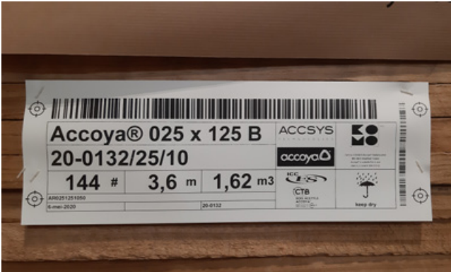
3.4 ACCOYA BUNDLE LABEL INCLUDING DIMENSION, GRADE, LENGTH, QUANTITY AND BATCH NUMBER
