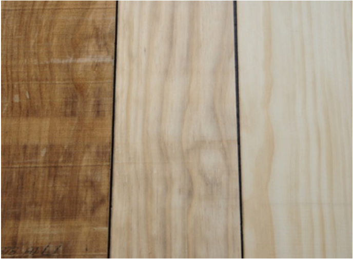
DISCOLOURATION: ROUGH BOARD, AFTER SURFACING 3MM AND AFTER SURFACING 6MM FROM ROUGH
