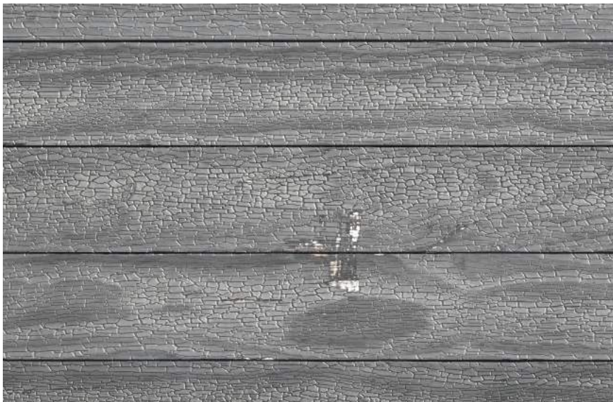
Damage from a ladder - scraped SSB Gator®
